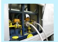
Each 15 m long, DN32 for max. oil temperature 90°C, in oil and vacuum-tight design. Flange connection on transformer side and quick coupling at the side of the plant.
