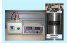
With the Tan delta Online measuring instrument it will be possible to measure actual value ether on the inlet or outlet of the plant. The Online measuring data's will be shown on the PLC Screen.
