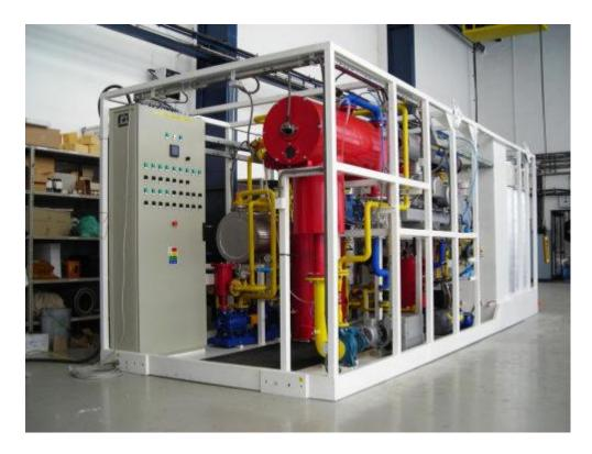
If the adsorption clay reaches its maximum saturation, the RU is automatically separated from the PU. While the PU is further on treating the oil (degassing, dehumidification and filtering), the RU starts to reactivate the saturated adsorbens. As soon as this process is completed, the RU is again connected with the PU for normal operation (treatment an regeneration).
