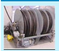
Electrical driven cable reel with 4 separate segments for 40m power cable of D 22mm.
